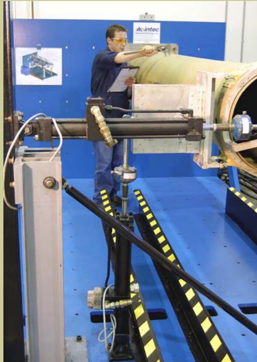
NOTAR TAILBOOM Static Multi-axis AS4/APC-2 Proof Test, 64 Strain Channels, Three Axis, 237% of Limit Load
