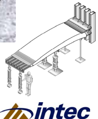
COMPOSITE WING BOX Static Aerodynamic and Internal Pressurization, 170” Long 60” wide, 20” deep, 5M in-lbs Reaction Fixturing, Four Axis, 379 Strain Gages, Internal Pressurization
